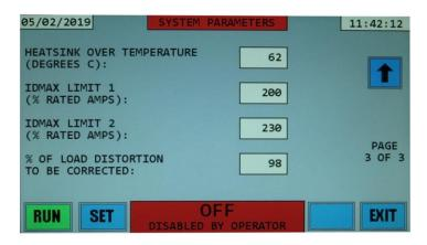
**HEATSINK OVER-TEMPERATURE (DEGREES C)** – If either of the two temperature sensors on the heatsink reaches the value shown here, the unit will shut down.
