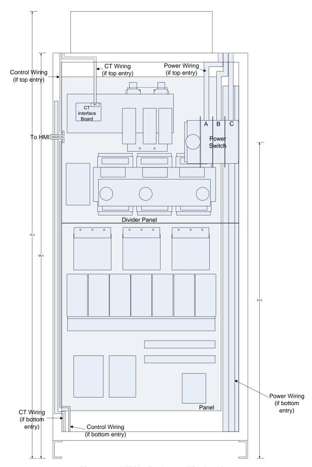
Figure 3.8: NEMA1 Enclosure Wire Routing
