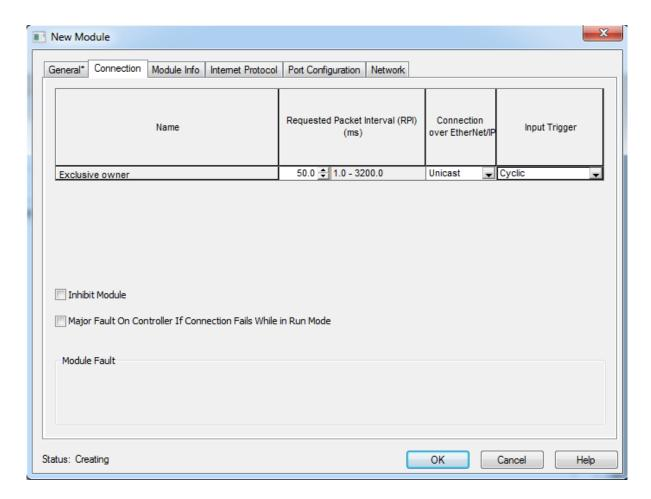
The default RPI is set to 50mS because this is approximately how fast the data is being updated by the Ethernet/IP module internally in the DPM. The Ethernet/IP Module is capable of delivering data as fast as 1mS, however keep in mind that the actual data will not change that fast. If necessary, you can also read the data as slow as every 3.2 seconds, this depends entirely on your application.
