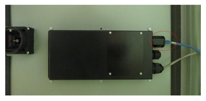
Your system is shipped with its Ethernet DHCP enabled. This will allow your network (or computer) to automatically assign an IP address to the DPM.
