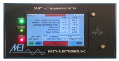
The Power LED is on and green when the HMI module has power. It is off when the HMI module does not have power. If you are having problems with the Front Panel LCD turning on, make sure that the Power LED is on, if not there is likely an issue with power going to the HMI Front Panel.
