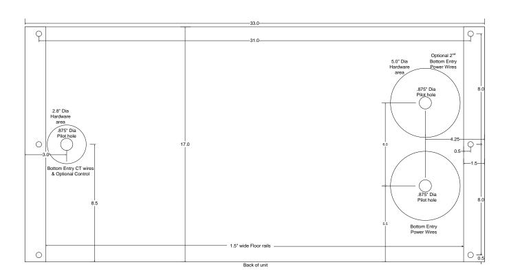
Figure 3.7: 300 Amp DPM NEMA1 Cabinet Bottom Wire Entry
