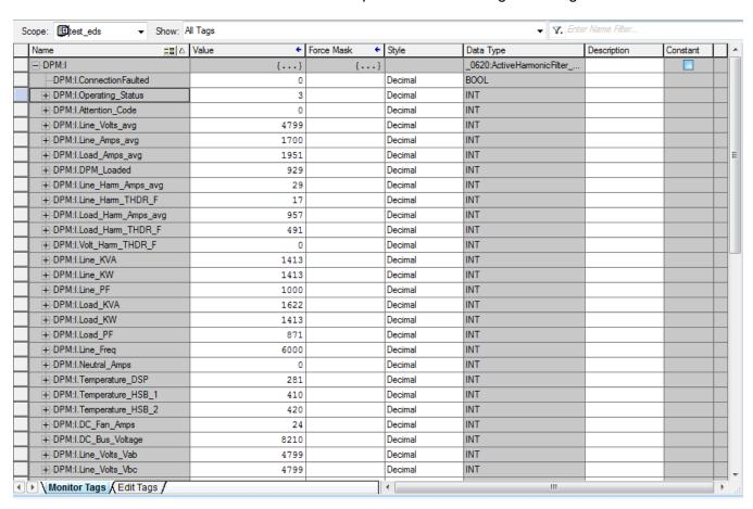
As you can see each data location has a corresponding name which matches the name in Table 7.2 in section 7.1 of this manual. Each location is an integer and can have a value between 0-32767.
