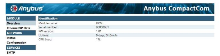
Click on Status under NETWORK to see more detailed network information. Click on Configuration under NETWORK to set a Static IP Address.
