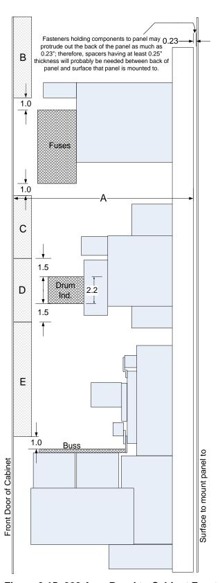
Figure 3.15: 300 Amp Panel to Cabinet Front Door Dimensions
