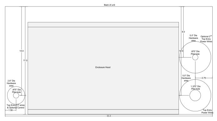
Figure 3.6: 300 Amp DPM NEMA1 Cabinet Top Wire Entry
