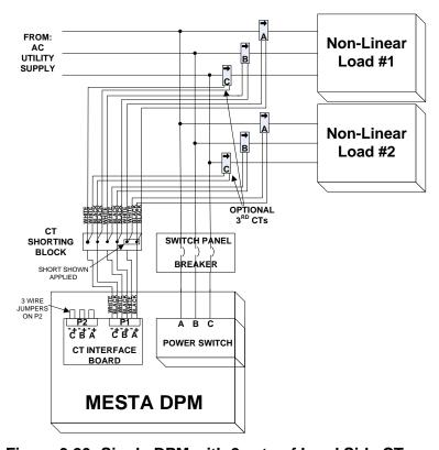
Figure 3.20: Single DPM with 2 sets of Load Side CTs monitoring 2 loads
