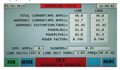
To enable the system, press the "RUN" button in the bottom left corner of the OPERATING STATUS LCD display page. This will result in the following display:
