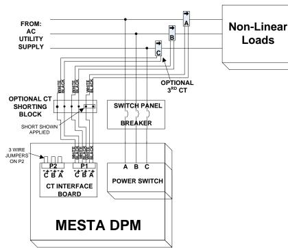
Figure 3.18: Single DPM with Load Side CTs monitoring one load
