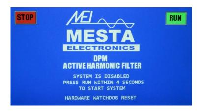
As can be seen in the example picture, the message "HARDWARE WATCHDOG RESET" is shown at the bottom of the display. Table 9.3 lists the possible HMI reset reason messages and actions to take to solve the issue.
