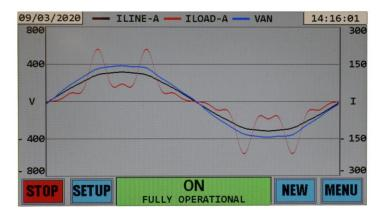
The three multicolored bars to the left of the waveform titles show what color is used to display each waveform. There are two separate grids, one for the voltages on the left with the letter V representing 0 volts, and one for the currents on the right with the letter I representing 0 amps. If only voltages are displayed, the grid on the right would not be displayed. Likewise, if only currents are displayed, the grid on the left would not be displayed.
