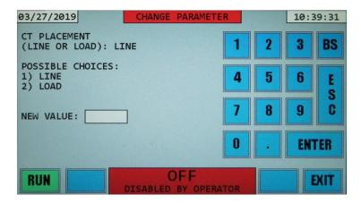
5. There is now a keypad on the right side of the display. At the top of the information section is the present parameter value, in our example "LINE". Below that are the possible choices for the parameter. In this example there are 2 choices Line or Load. Entering 1 will choose Line for the new value, entering 2 will choose Load for the new value. Entering any other number will result in the error message "BAD INPUT – TRY AGAIN" being displayed.
