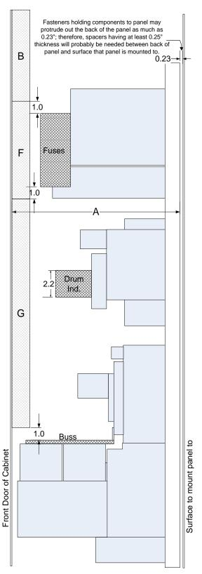
Figure 3.14: 50-200 Amp Panel to Cabinet Front Door Dimensions
