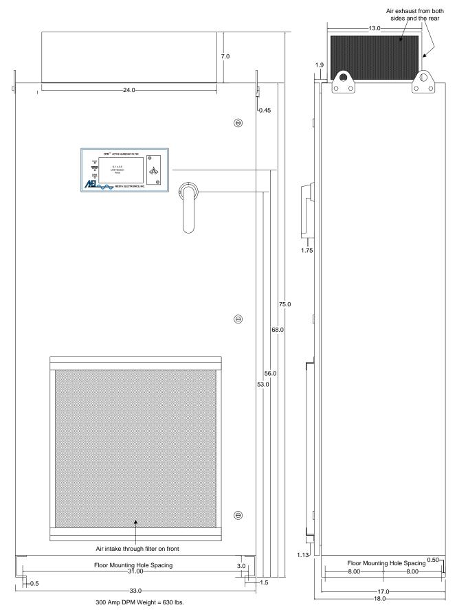
Figure 10.8: 300 Amp NEMA1 Enclosed DPM Drawings
