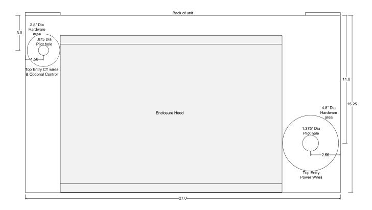
Figure 3.4: 150 or 200 Amp DPM NEMA1 Cabinet Top Wire Entry
