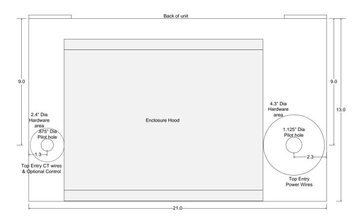
Figure 3.2: 50 or 100 Amp DPM NEMA1 Cabinet Top Wire Entry
