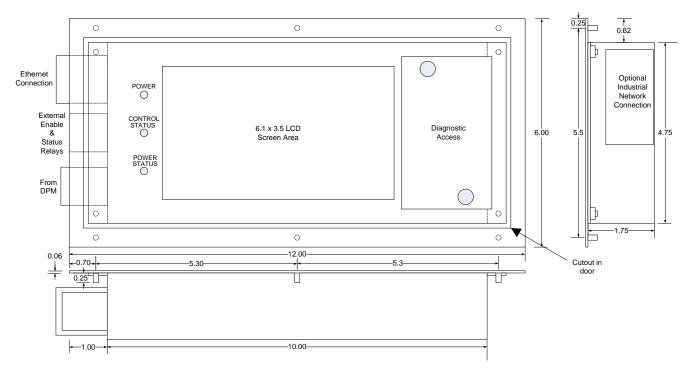
Figure 3.13: HMI Dimensions
