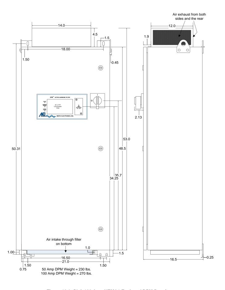
Figure 10.6: 50 & 100 Amp NEMA1 Enclosed DPM Drawings
