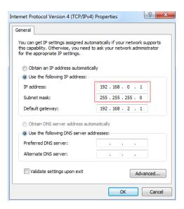
Select "Use the following IP address:" and type in 192.168.000.001 for the IP Address and 255.255.255.000 for the Subnet mask. It doesn't matter what the Default Gateway is. These are circled red in the picture above.
