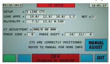
Please note that the button on the lower left is blank and should be green. The button is blank and non-functional to prevent the unit from being enabled while in the CT SETUP display. If the unit was already enabled, the button on the bottom left would be red and say STOP.
