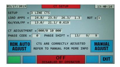
To remove a CT adjustment, press the REM.AUTO ADJUST button.
