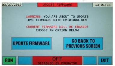
This screen gives a warning that you are about to erase the current HMI firmware and replace it with HMI01000.BIN and gives you a choice to proceed by pressing the UPDATE FIRMWARE button, or to go back and select another file by pressing GO BACK TO PREVIOUS SCREEN. You can also press EXIT to go back to the DIAGNOSTICS display.
