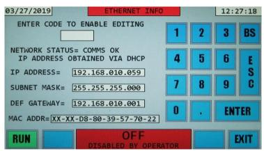
At the top of the information section it says ENTER CODE TO ENABLE EDITING. This is used to enter the display for changing the IP address mode: Static IP Address or DHCP IP Address. This will be covered in section 5.9.1.
