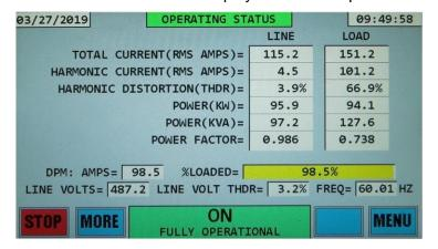
There are 2 columns in the "informational section", one for the LINE information and one for the LOAD information. All values on this screen except for frequency and power are averages of the three phases.
