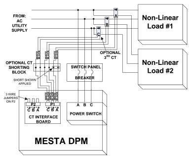
Figure 3.19: Single DPM with 1 set of Load Side CTs monitoring 2 loads
