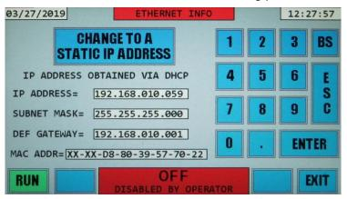
Press the CHANGE TO A STATIC IP ADDRESS button. This button will now say CHANGE TO A DHCP IP ADDRESS. The values next to IP ADDRESS, SUBNET MASK, and DEF GATEWAY now have blue rectangles around them which indicate that these are buttons. See the following picture.
