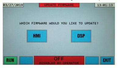
5. The factory will inform you if you need to update the HMI or DSP firmware. Press the appropriate button HMI or DSP. In our example we will press the HMI button. The following screen will open. See picture below.
