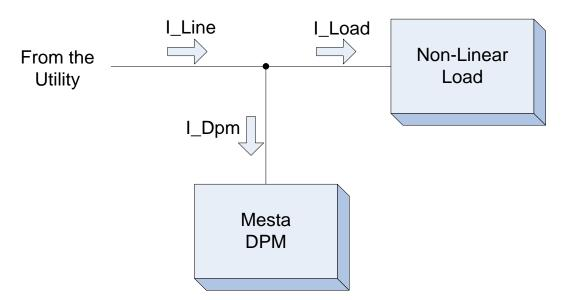
Figure 1.1: Simplified 1-line Diagram of a DPM Installation
