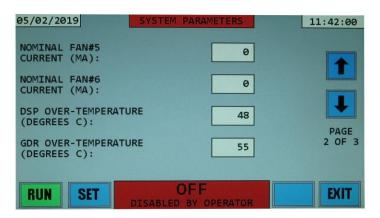
As mentioned earlier, the first 2 value on this 2<sup>nd</sup> page are the nominal currents for FAN#5 and FAN#6. FAN#5 will be zero for all units except for a Nema1 300 amp system. FAN#6 output is presently not used in any systems, so will always be zero.
