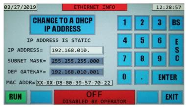
The period key is disabled in this screen. Now in our example we enter 060 with the keypad. After pressing Enter, the rectangular area around IP ADDRESS became blue again, and the IP Address inside this area is now 192.168.010.060 as shown in the following picture:
