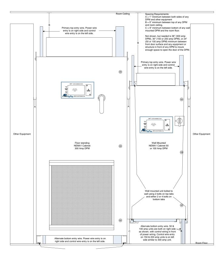
Figure 3.1: Installation Showing Clearances and Wire Entry
