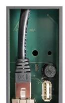
There is a front cover to the right of the LCD display that is attached with 2 thumb screws. Unthread the top screw, then just loosen the bottom screw so that you can swing the front cover open, exposing the components as shown in the picture to the right. The USB connector can be used to plug in a flash drive. The HMI via the LCD display can be instructed to download various stored history data to the drive (see section 5.8 for additional details).
