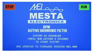
As an additional verification you can open the CONFIGURATION PARAMETERS DISPLAY as described in section 5.6.4 and verify that the HMI Software version matches the version number of the file. In our example we updated the HMI firmware with HMI01000.BIN, and in the CONFIGURATION PARAMETERS display the HMI Software Version is 001.000. See picture below.
