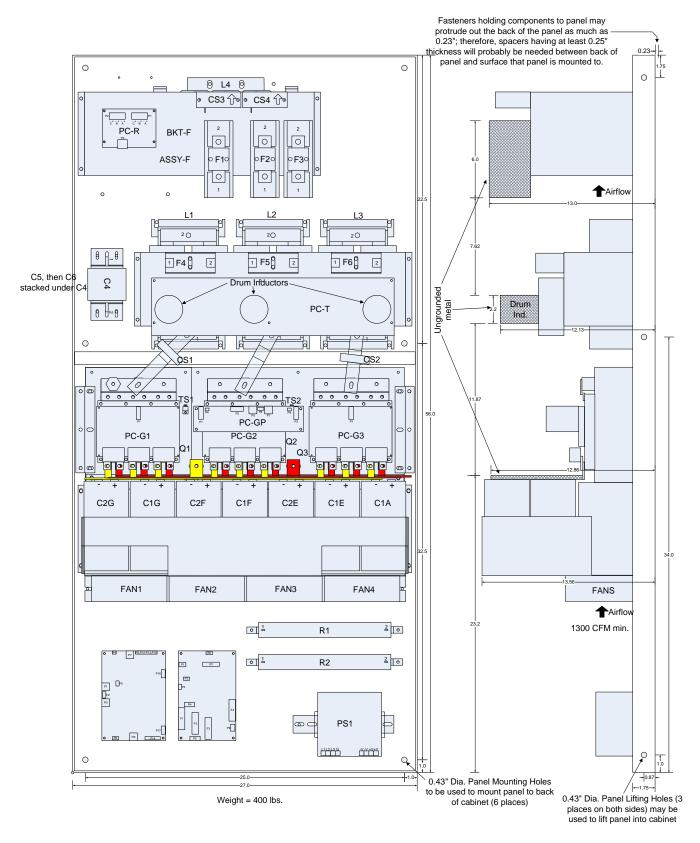
Figure 10.5: 300 Amp DPM Panel Layout Drawings
