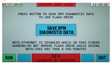
First make sure that a USB flash drive is inserted into the USB port on the front panel. The flash drive USB port is located under the protective cover to the right of the LCD screen on the front panel of the HMI. Refer to section 3.5.6 on opening the cover and locating the USB port.
