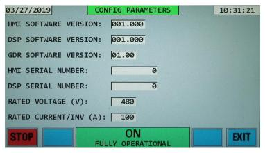
In this display the operator is able to view configuration parameters such as: DPM Software versions, DPM Serial Numbers, as well as the system Rated Voltage and Rated Current.
