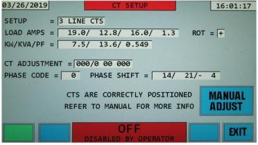
This display is very useful in determining if the external LINE or LOAD placed current transformers (CTs) are placed on the correct phases and in the correct direction. Section 4 of this manual covers how to use this display to check the placement of the CTs.
