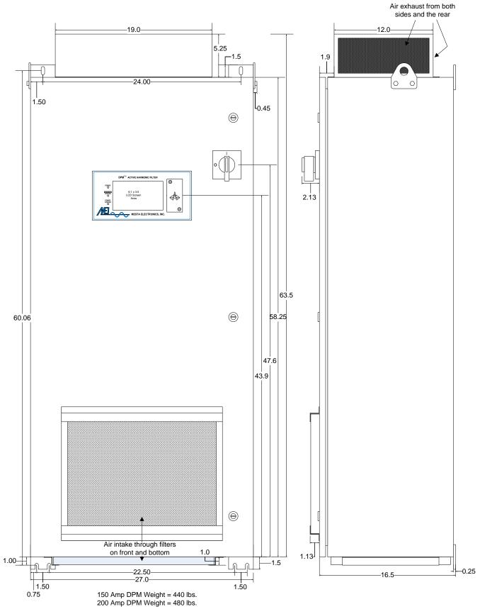
Figure 10.7: 150 & 200 Amp NEMA1 Enclosed DPM Drawings
