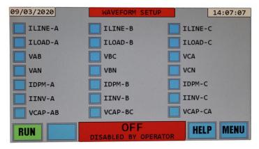
There are 21 parameters which can be viewed. There are 7 rows, each row showing the parameters for phases A,B,C.
