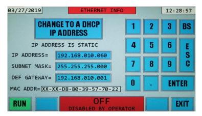
If needed, the subnet mask and default gateway can also be altered; however that is not necessary for this case. When done, press the EXIT button.
