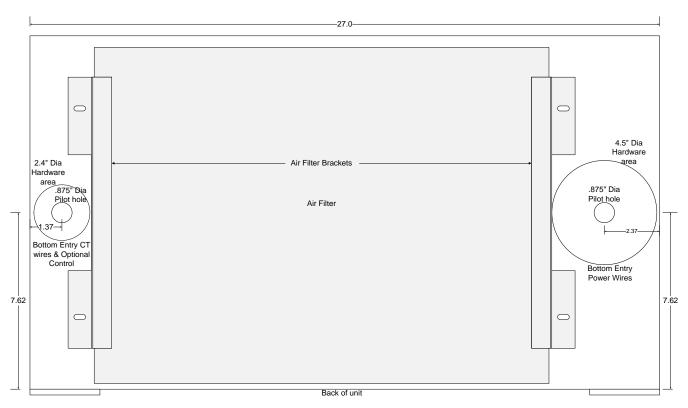
Figure 3.5: 150 or 200 Amp DPM NEMA1 Cabinet Bottom Wire Entry
