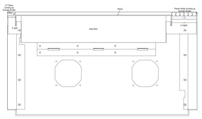
Figure 3.11: 300 Amp DPM NEMA1 Wire Passage Through Divider Panel
