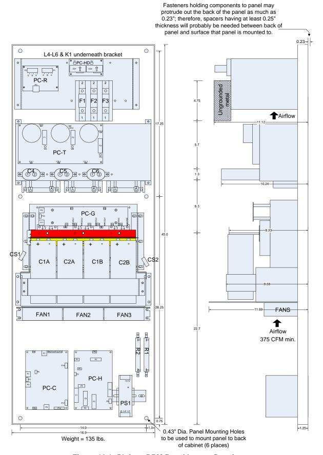
Figure 10.1: 50 Amp DPM Panel Layout Drawings
