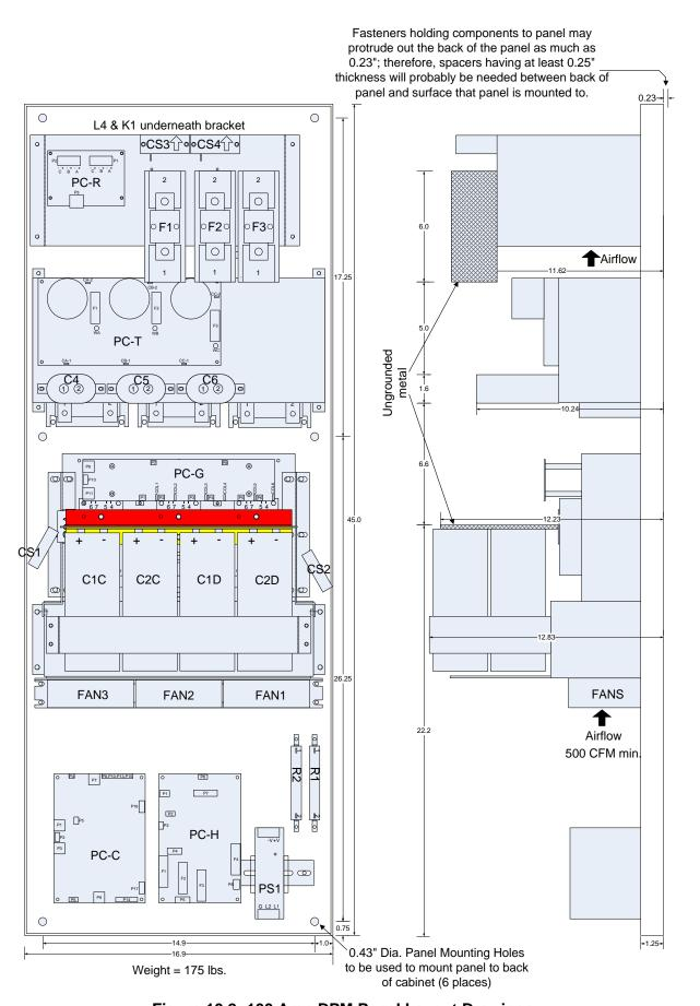
Figure 10.2: 100 Amp DPM Panel Layout Drawings
