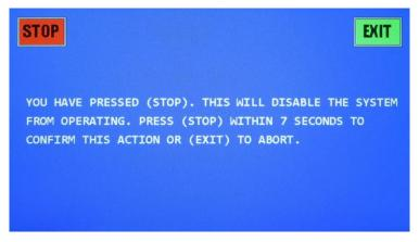
The red "STOP" button on this display will have to be pressed before the 10 second timer on this display expires, for the system to become disabled. Pressing the "EXIT" button on this display will result in immediately going back to the previous display without disabling the system. Once a system is disabled, a green "RUN" button will appear on all "Status" sections of displays in place of the red "STOP" button. Disabling a system will immediately stop a system from running.
