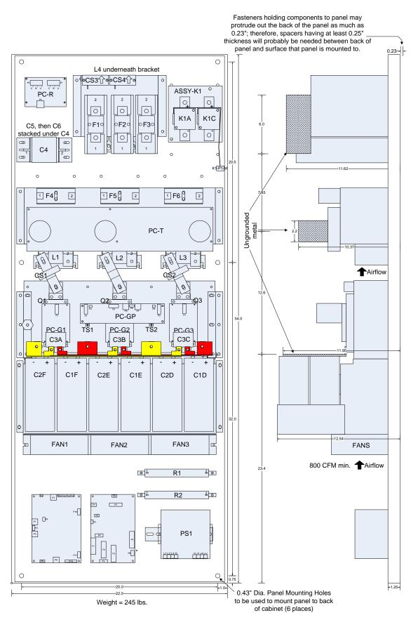
Figure 10.3: 150 Amp DPM Panel Layout Drawings
