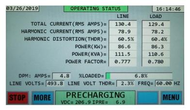
Note that once the DPM is told to RUN, the place where the RUN button was previously located, there is now a STOP button. Since the DPM is already "running", there is no need to command it to run; however, now there may be a need to "stop" or disable the DPM from running; hence a STOP button is provided to allow that action.
