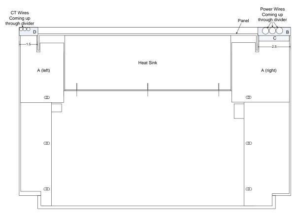
Figure 3.9: 50 or 100 Amp DPM NEMA1 Wire Passage Through Divider Panel
