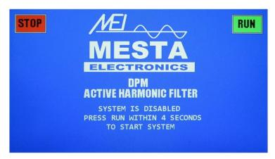
**Do not press RUN when powering on the unit for the first time.** After 5 seconds the "OPERATING STATUS" display page will appear. Pressing the STOP button when the splash screen is displayed will immediately send you to the "OPERATING STATUS" display instead of waiting the 5 seconds.
