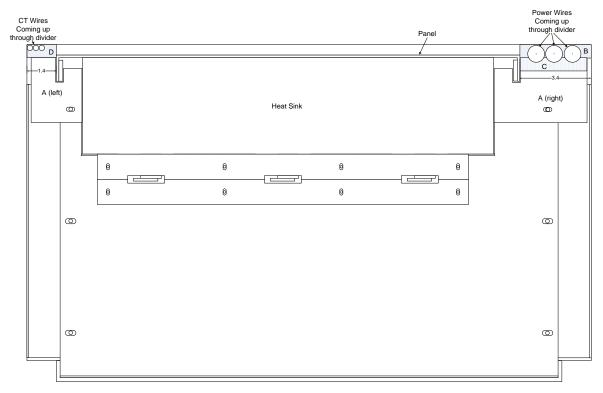
Figure 3.10: 150 or 200 Amp DPM NEMA1 Wire Passage Through Divider Panel
