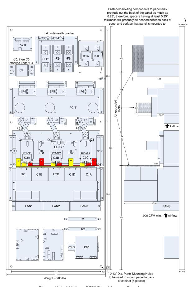
Figure 10.4: 200 Amp DPM Panel Layout Drawings
