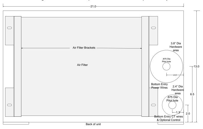
Figure 3.3: 50 or 100 Amp DPM NEMA1 Cabinet Bottom Wire Entry
