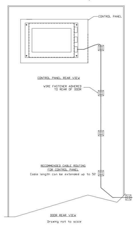
Figure 3.16: Possible Routing Path for HMI to PC-C Signal & Power Cat 5 Cable
