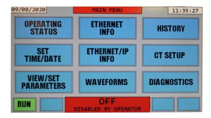
Note: your system may not have Ethernet/IP or Modbus TCP capability. In that case the button which says ETHERNET/IP INFO in the picture above will say INDUSTRIAL NETWORK and be grey and inactive. See section 7 for information about the industrial network option for the DPM.
